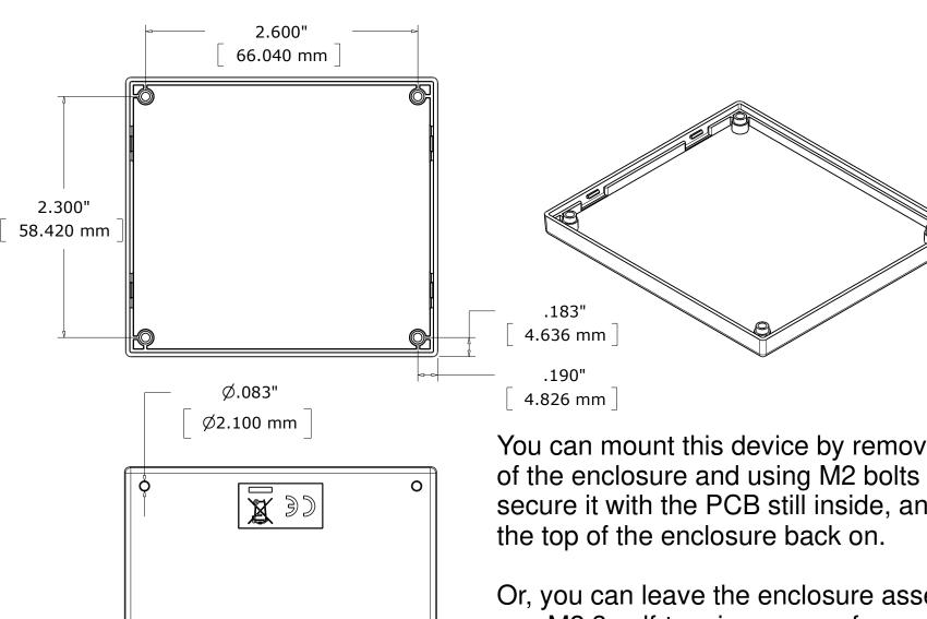
You can mount this device by removing the top half of the enclosure and using M2 bolts and nuts to secure it with the PCB still inside, and then snap
