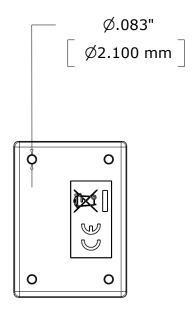
You can mount this device by removing the top half of the enclosure and using M2 bolts and nuts to secure it with the PCB still inside, and then snap the top of the enclosure back on.
